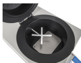
Chamber for moisture content determination of special design
